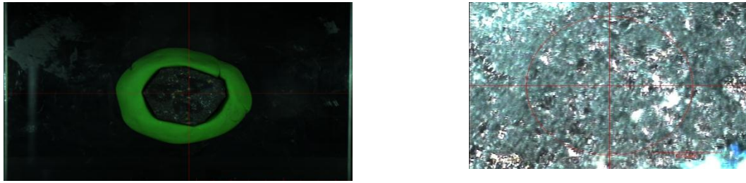
Figure 20 Sample-(A2b). XGT photomicrograph of Cr with Mg, Fe, Al and Pm (promethium).
