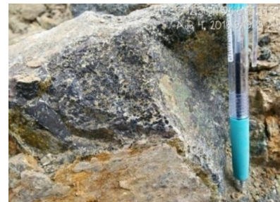
Figure 15 Massive ore (Tiger ore) has more chromite than Leopard ore in the study area.
