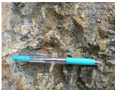
Figure 7 Spotted type chromitites formed by partially or totally fill the interstices between olivine grains at Saisaquine worksite.
